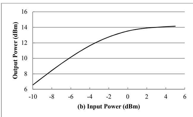
Fig. 10. Output Power and PAE vs. Input Power. (a) in percent and (b) in numerical values.
