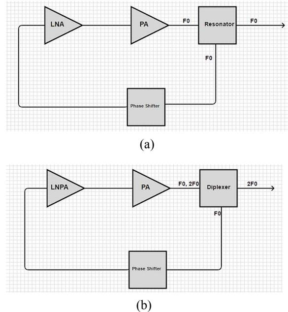
Fig. 4. Feedback Oscillator Diagram: (a): Conventional, (b): Harmonic
