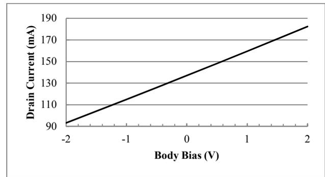
Fig. 5. Drain Current with Respect to Body Bias
