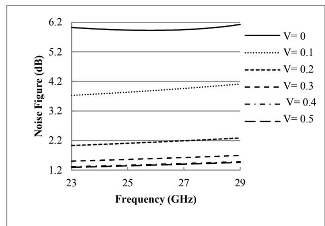
Fig. 6. Noise Figure at Different Biasing
