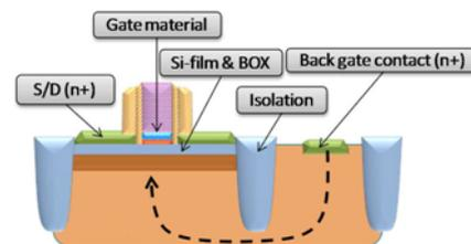
Fig. 1. UTBB FD-SOI Geometry
