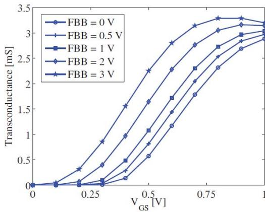
Fig. 3. Impact of FBB on Transconductance [4]
